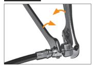
STEP 1: Installing a connector requires two wrenches - one for the hose and a second for the fitting. The wrench size for the hose is 14 mm. The wrench size for the fitting depends on the fitting.
